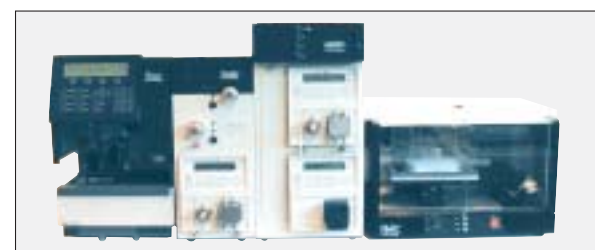
Figure 2. UltiMate ™ capillary/nano LC system with Probot: from left to right a FAMOS ™ micro autosampler, Switchos ™ micro-column switching module, UltiMate micropump and detection module, and Probot.
